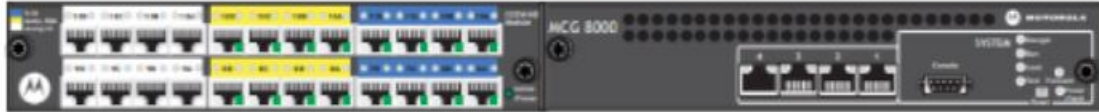
Figure 3 Enhanced MCG 8000 Conventional Channel Gateway—Connects dispatch operators to analog or digital conventional channels in the system.
