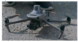
**Capability:** The DJI Mavic 30T Enterprise series is a remote piloted drone with about 41 minutes of max flight time, capable of live video capture that can be displayed to the pilot.
