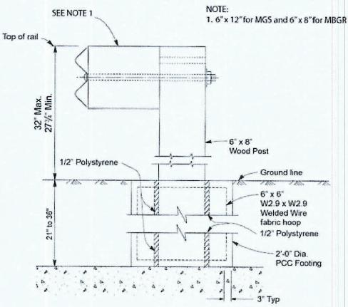
Form socket in concrete to receive 6" x 8" post or place concrete around 6" x 8" post wrapped with one layer of 1/2" thick expanded polystyrene foam sheeting. Do not nail polystyrene to post. Post to be centered in concrete footing.
